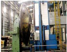
• Up to  $12.9 \text{m} \times 3.9 \text{m}$  high  $\times 2.0 \text{m}$  Z travel.
